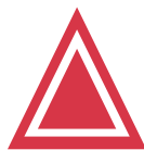
Figure 2.11 – Balise de tribord
